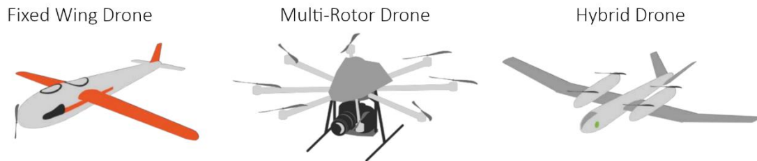
Figure 3: The three types of drones, from left to right, fixed-wing, multi-rotor, and hybrid. Picture(s) retrieved from Swiss Foundation of Mine Action and CartONG (2016a, p. 17)
