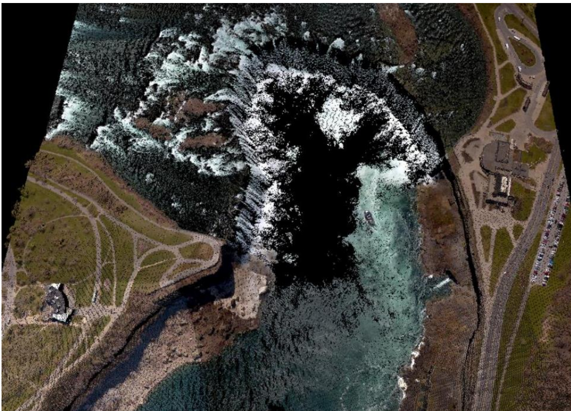
Figure 8: Colorized point cloud collected using lidar. Black spots are missing data. Image retrieved from Simmers and Wagg (2013, p. 4)
