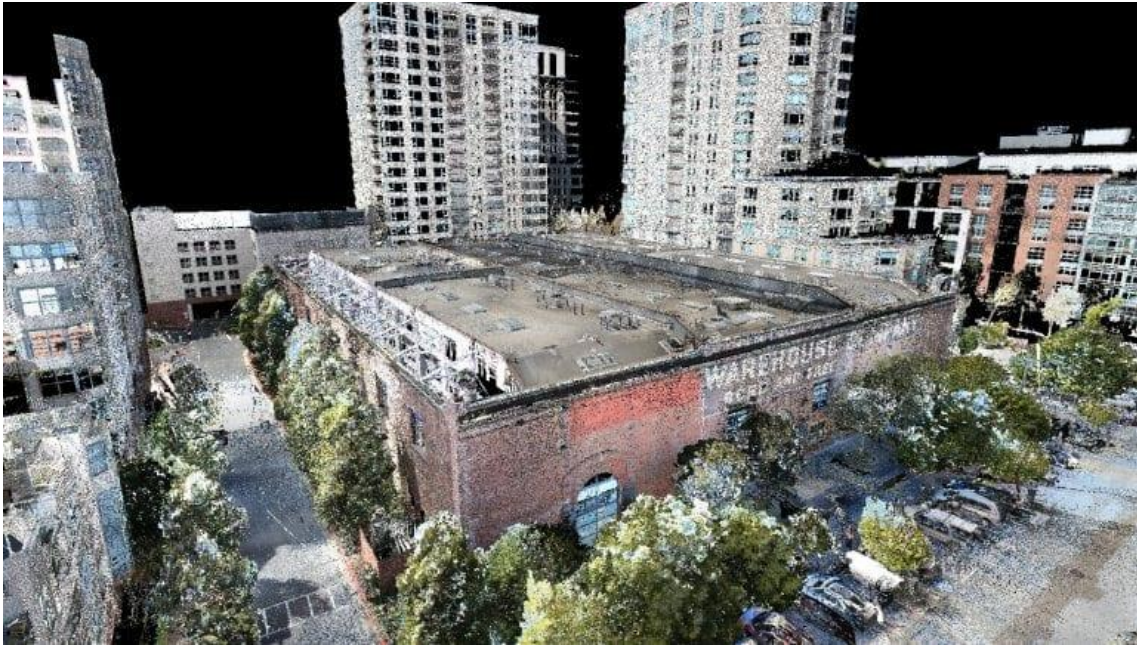
Figure 5: An example of a 3D model of a warehouse and surrounding buildings made using photogrammetry. Image retrieved from Jobsite Editorial Staff (2018)
